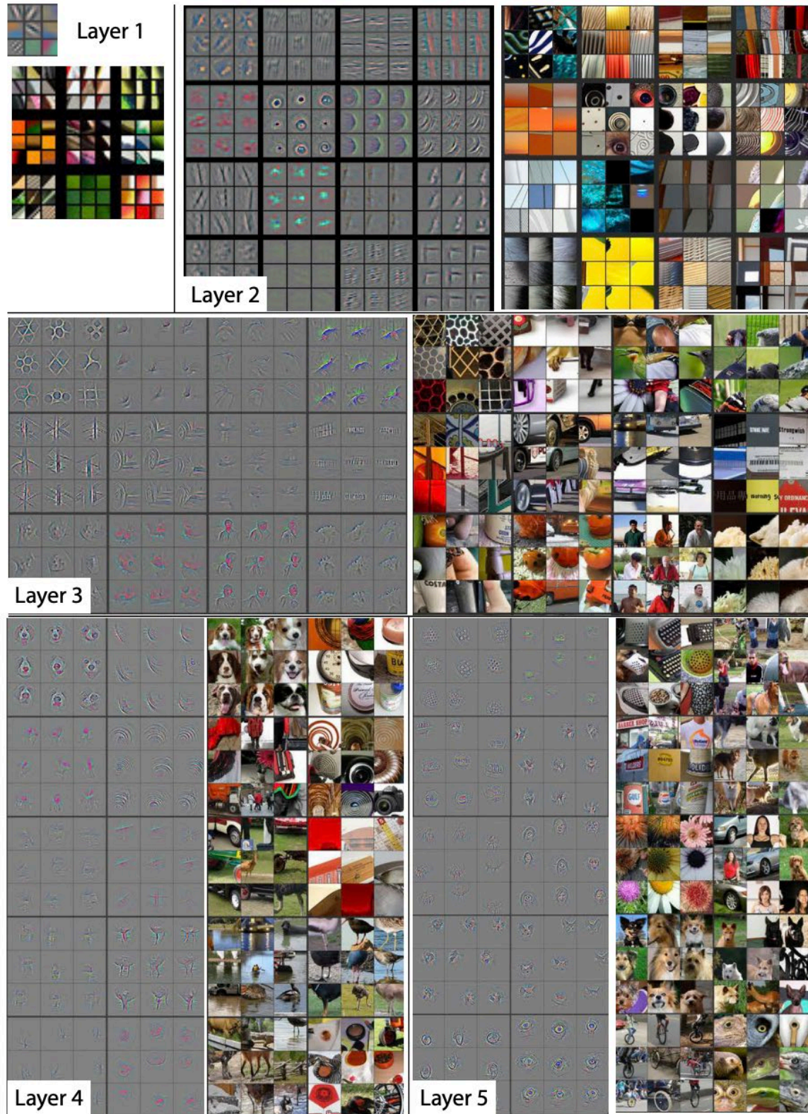
Figure 2.14: Visualization of features in convolution layers of a trained network (Zeiler & Fergus, 2014)
