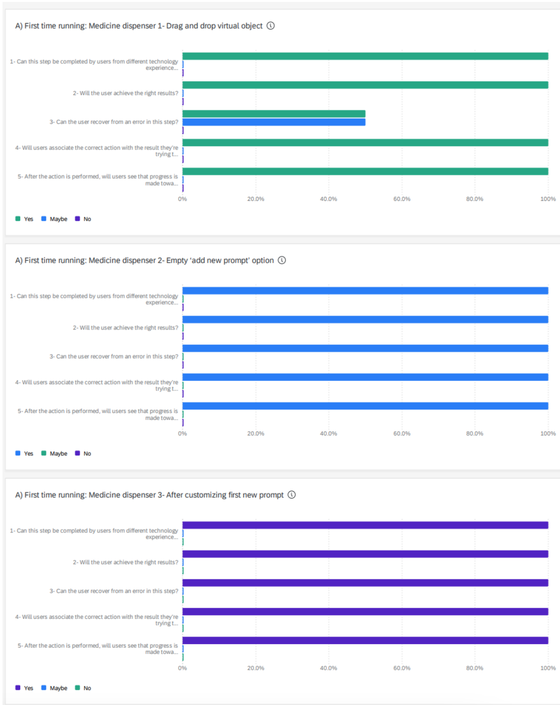
Figure E.6: A screenshot of the cognitive walkthrough row data as exported from Qualtrics. The screenshot is taken from caregiver user mode evaluation. As shown, each system event is inspected using five questions. Evaluators answered the same set of questions for all user tasks / system events
