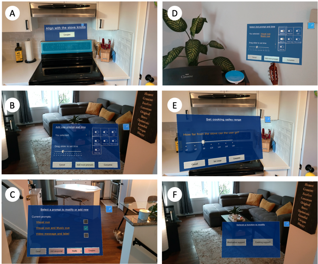
Figure 9.2: Sample of the caregiver mode user interface screenshots. A) shows the caregiver aligning the virtual object with the stove. B) the caregiver is adding a new prompt. C) modifying existing prompts, D) customizing a prompt. E) setting cooking safety range. F) selecting a function
