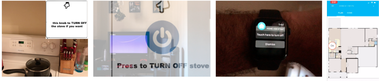
Figure 6.8: Screenshots of the video prototype. a) Memory prompts showing the user how to turn off the stove, b) virtual button, c) the user receives a message on Apple Watch when taking off MR glasses, D) screenshot of the caregiver mobile app
