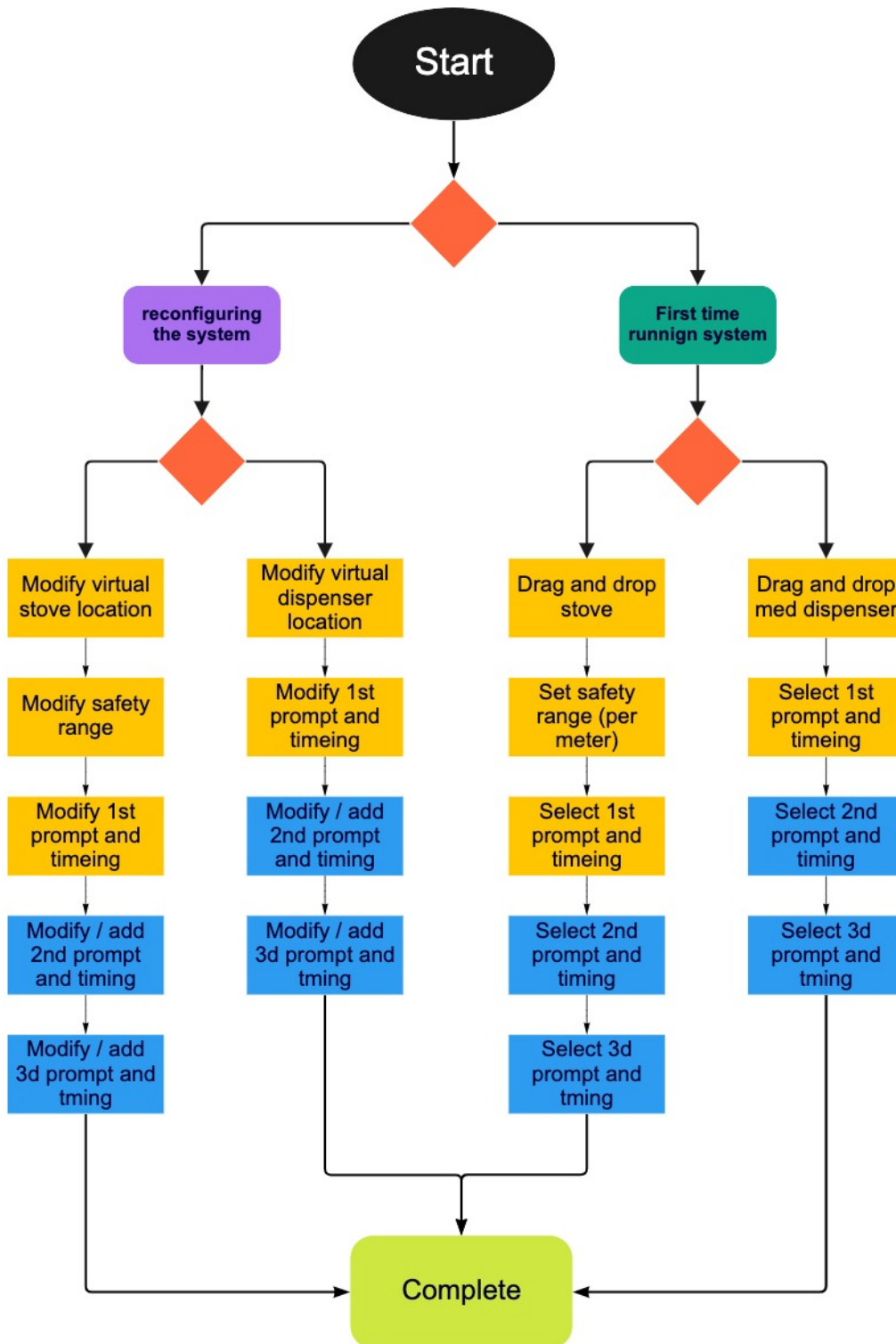
Figure E.5: Caregiver user flow diagram presenting all user tasks for setting up the system first time and for reconfiguring. Yellow coloured tasks are required while blue coloured tasks are optional
