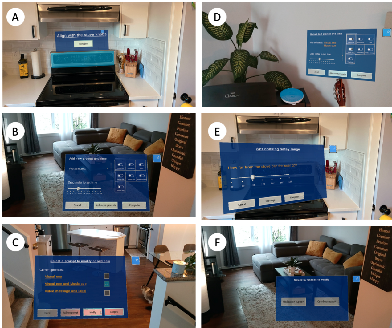
Figure E.4: Sample of the caregiver mode user interface screenshots. A) shows the caregiver aligning the virtual object with the stove. B) the caregiver is adding a new prompt. C) modifying existing prompts, D) customizing a prompt. E) setting cooking safety range. F) selecting a function
