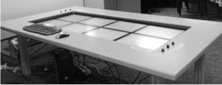
Fig. 1. The 183cm x 122 cm digital tabletop with 10 mega pixels output resolutions
