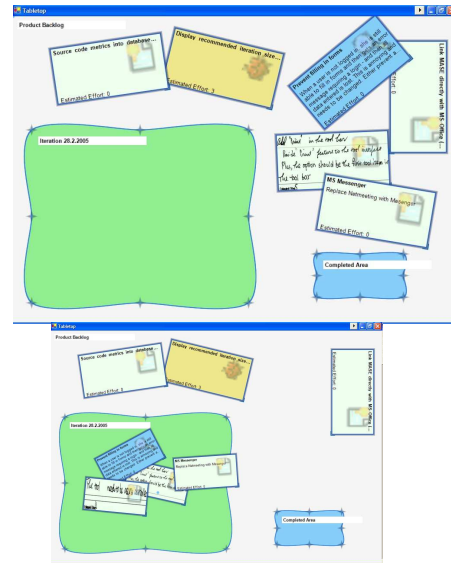
Figure 8: The local and shared images of the Planning Area in private mode: displayed on the tabletop (top panel, visible to the whole team) and on the Tablet PC of a single user (bottom panel, visible only to the Tablet PC user).
