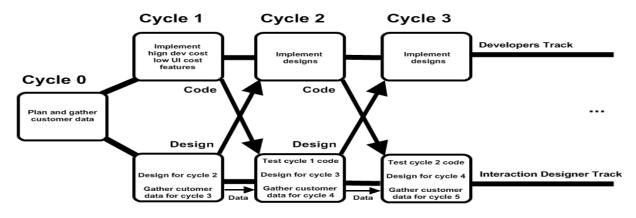
Fig. 1. Sy's interaction designer/developer tracks diagram
