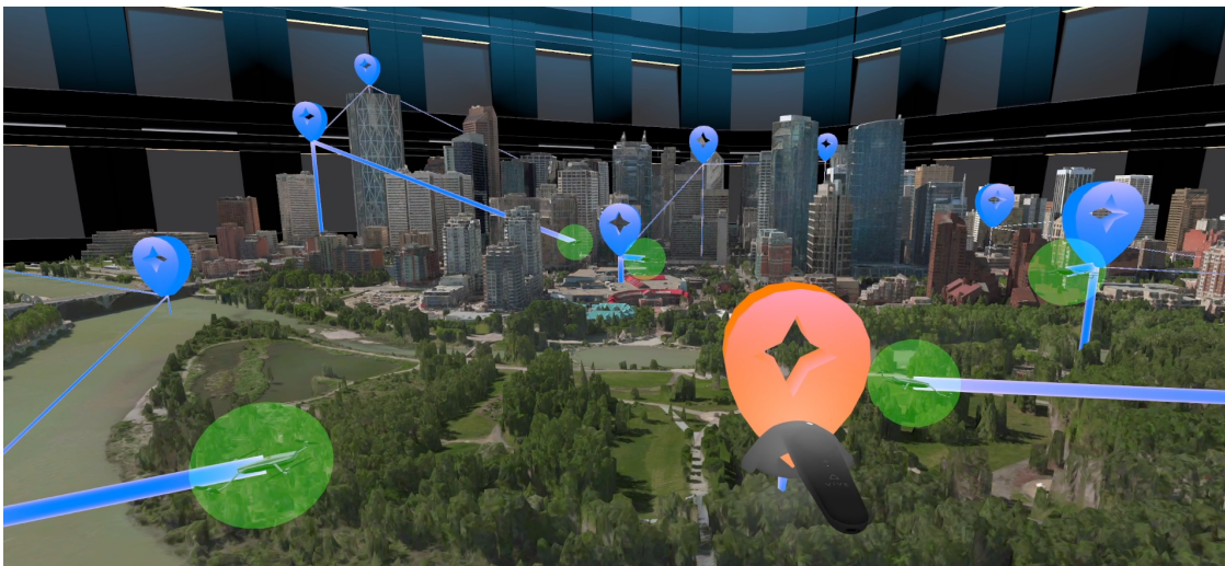
Fig. 4. A large-scale view from within the 3D GCS map of Calgary, Canada from Figure 3. To achieve this viewpoint of the operating environment, the user has scaled the map up to the size of a small room, placed themselves inside of it, and is currently in the process of manually placing a waypoint on the map with their controller.
