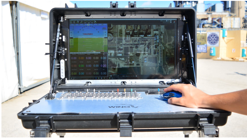
Fig. 2. Worthington Sharpe's Wing GCS [12], an example of a mobile GCS used for deployment in outdoor operational environments.
