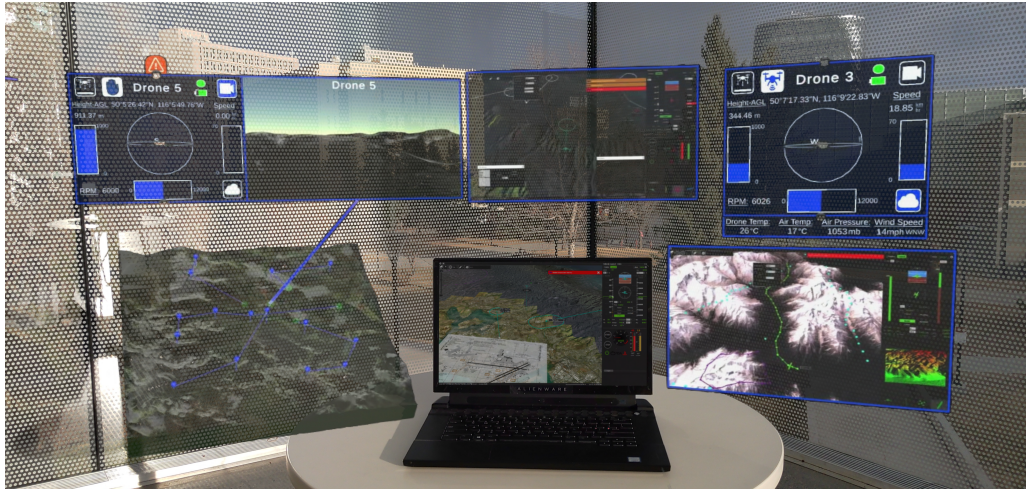
Fig. 1. An example of what a cross-reality GCS experience could look like. Here a conventional GCS controlling UAVs from a remote location is run on a laptop (bottom-center) and is paired with a mixed reality headset to expand its capabilities to display extra virtual screens (upper-middle & bottom-right), UAV information panels (upper-right & upper-left), and a 3D map of the operational environment (bottom-left). Images on the laptop and virtual screens are of the VCSi GCS by Lockheed Martin [8].
