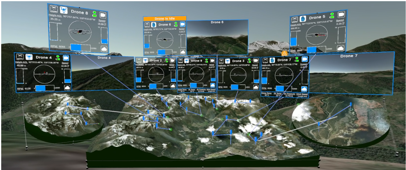
Figure 1: An extended reality ground control station workspace made up of a collection of 3D maps and robot information panels. Visualized on the three maps, one sees different perspectives of the operating environment for multiple aerial drones (highlighted in green) and their assigned flight paths (in blue) from varying zoom levels.
