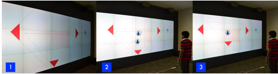
Fig. 3. Calibration. (1) Manually align the Kinects to overlap (2) A user stands in the overlapping area (3) Calibrate button is clicked on MSE Visualizer to calibrate the Kinects
