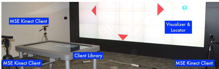
Fig. 1. MSE Architecture. Example environment with multiple MSE Kinect clients running, a tabletop running a client library and the MSE Visualizer and Locator service running on a wall display
