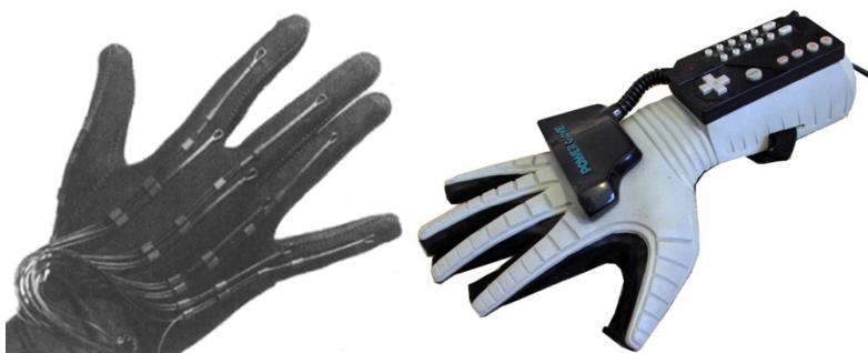
Figure 9: Data gloves such as the VPL DataGlove and Mattel Power Glove have been used since 1977 as hand gesture input devices.
