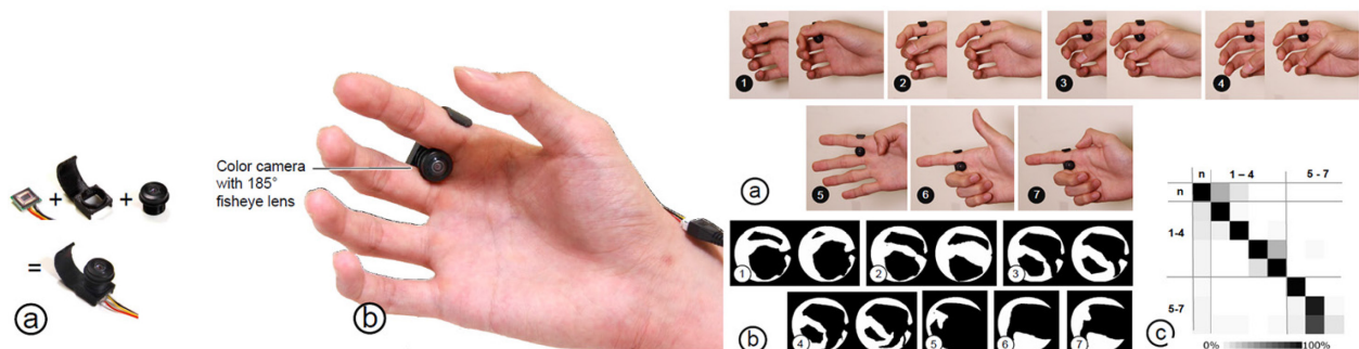
Figure 13: The CyclopsRing device uses a color camera with a fisheye lens to detect hand gestures (left). It was tested with a variety of hand gestures, many of which can be classified as SHMGs (right) [3].
