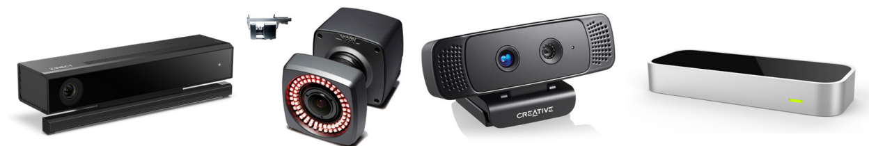
Figure 10: Visual gesture recognition devices such as the (from left to right) Kinect for Windows v2 [27], Vicon MX-F40 [54], Creative Sens3D [6], and the Leap Motion [23] often use infrared cameras. (Images are not to scale.)
