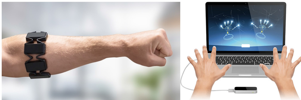
Figure 7: The Myo armband (left) detects hand gestures through electromyographic (EMG) sensors [51], while the Leap Motion (right) relies on infrared stereo cameras [23].
