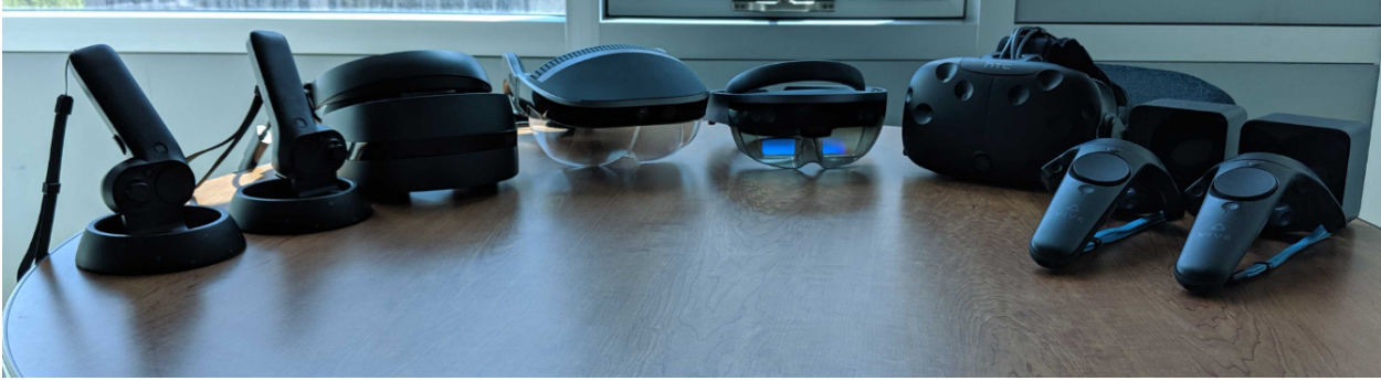
Figure 4.7: Picture showcase a range of different HMD XR product. From left to right: HP windows mixed reality headset with inside-out tracked controllers, Meta 2 with built-in hand tracking, Microsoft HoloLens with gesture controls, HTV Vive with base station tracking. All these devices have differences that should be considered when designing for them.
