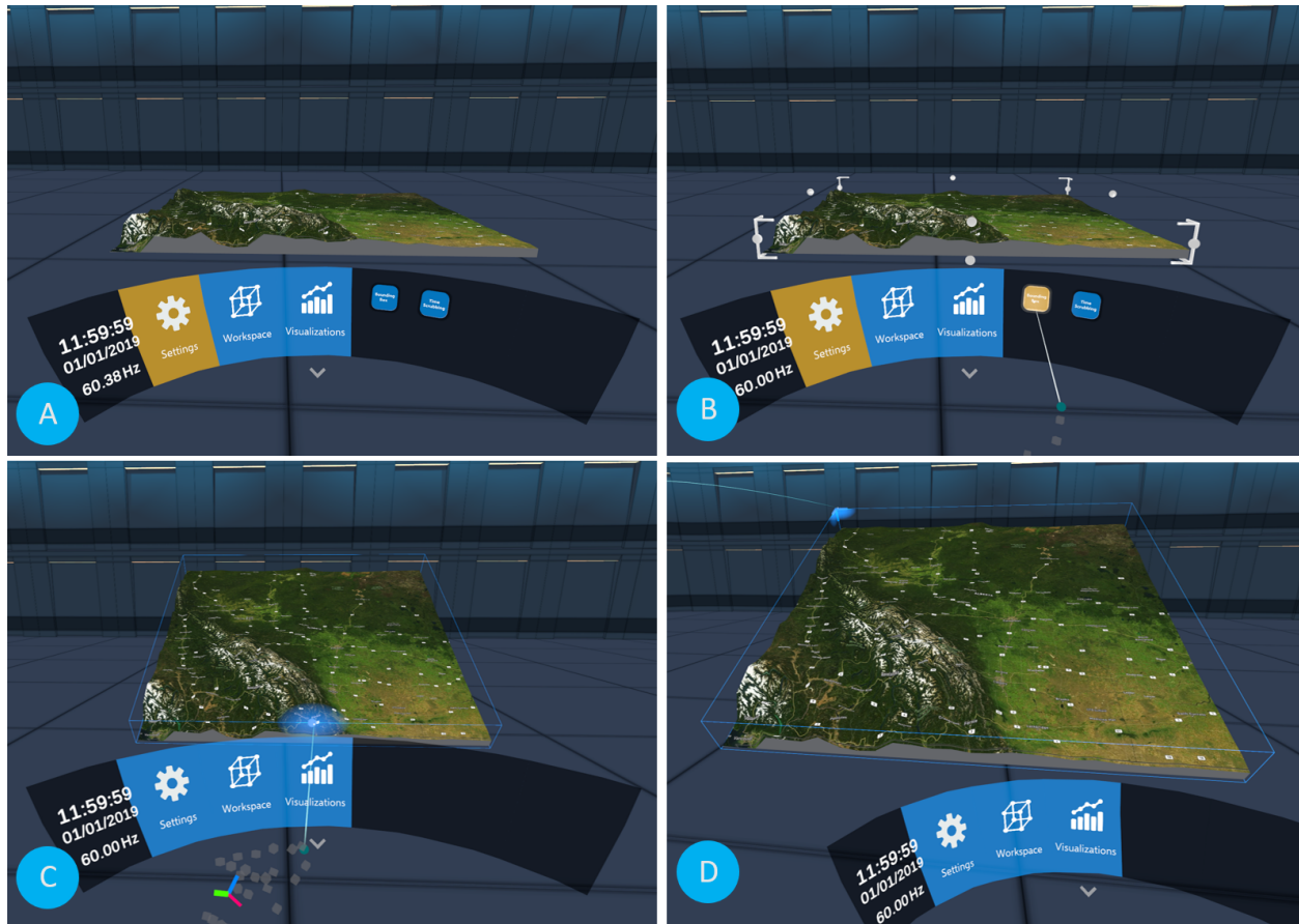
Figure 5.11: Shows the bounding box functionality. A: Map Visualizations with bounding box feature turned off. B: Bounding box feature turned on. C: Grabbing the circle allows the visualizations to be rotated on the corresponding axis D: Grabbing the corner allows for the visualizations to be scaled in the corresponding direction.
