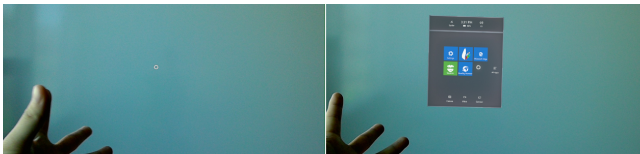
Figure 4.5: Microsoft HoloLens can toggle between showing and hiding the main menu through a bloom gesture.
