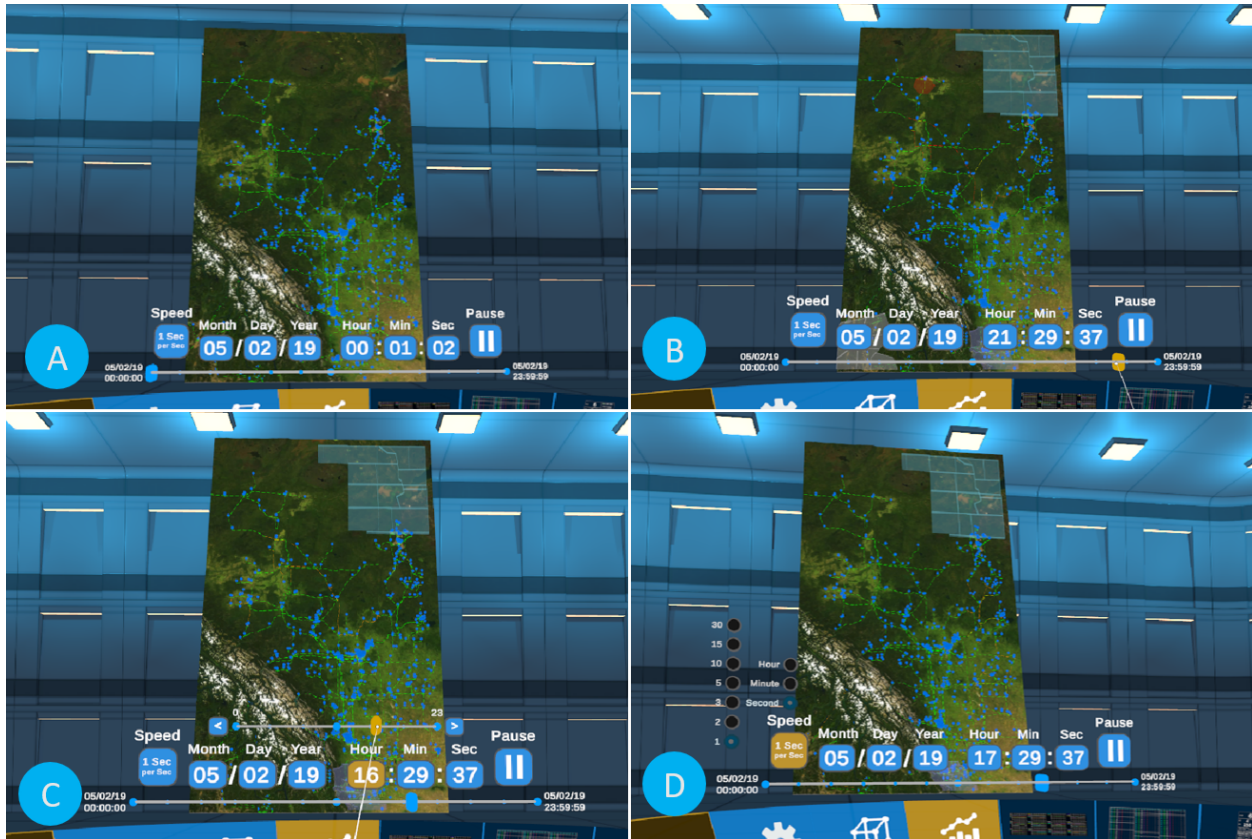
Figure 5.20: Time scrubbing functionality. A: Default time scrubbing menu. B: Changing the time through the main slider. C: Changing a specific time unit through a micro scrubber. D: Changing the playback speed.
