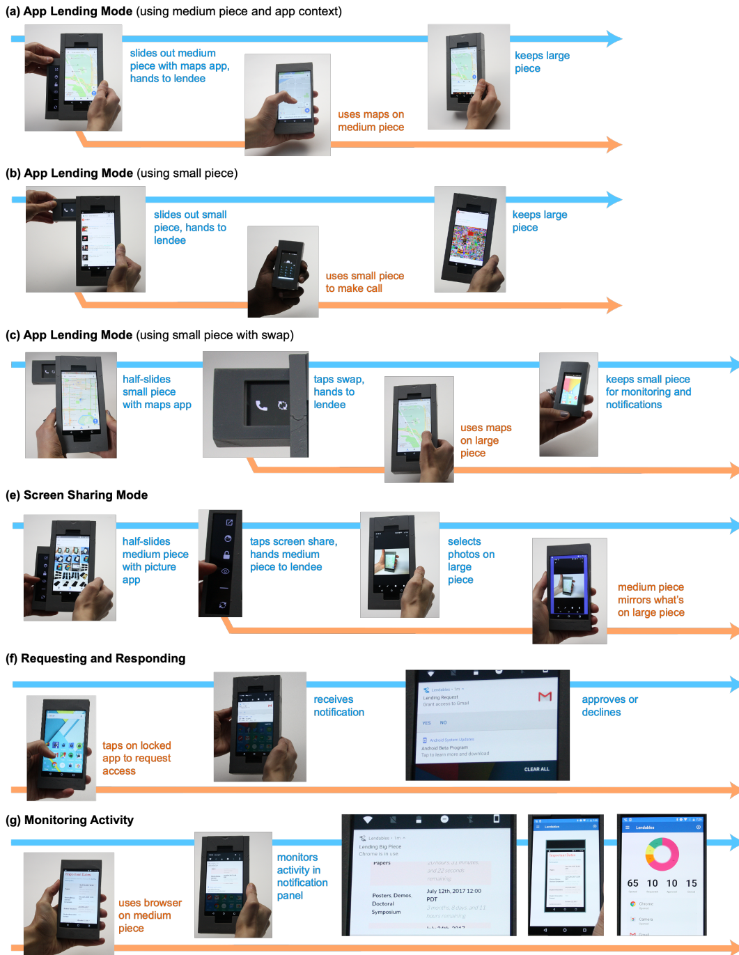
Figure 37: Interaction design flows showing lender interactions on blue line and lende interactions on orange line. Refer to text for detailed explanation and see the accompanying video for demonstrations of these interactions.
