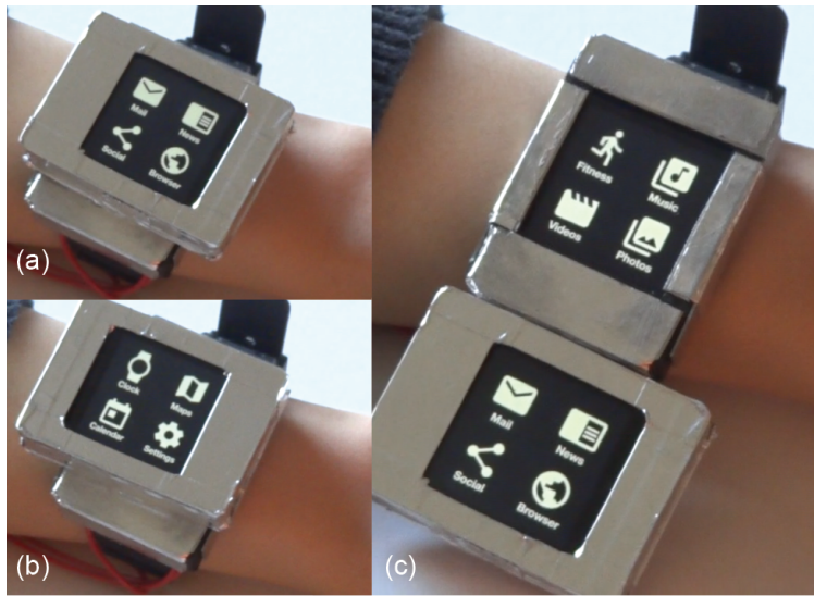
Figure 28: Launching apps: (a, b) frequent app icons in left and right groups; (c) viewing more app icons in group.
