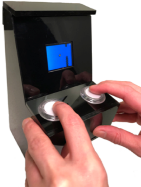
Figure 49: An example of a completed MakerArcade system in the form of a miniature Arcade Cabinet running a user-created Flappy-bird like game with a default set of buttons mapped. This game (and others) can be mapped to different sensors (like an accelerometer) that a user can program and map as an alternative controller that is plugged into the cabinet which contains a headphone jack and uses our custom headphone jack-based hardware protocol.
