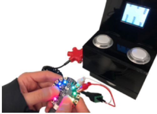
Figure 53: Buttons from an Adafruit Circuit Playground Express (CPX) used as a controller for the Flappy-bird game. The CPX is coded using blocks (and a custom plug-and-play headphonejack bus protocol) within MakeCode Maker. On MakeCode Arcade, a user simply programs additional buttons using our packages, which are auto-detected when plugged into the headphone jack hub.
