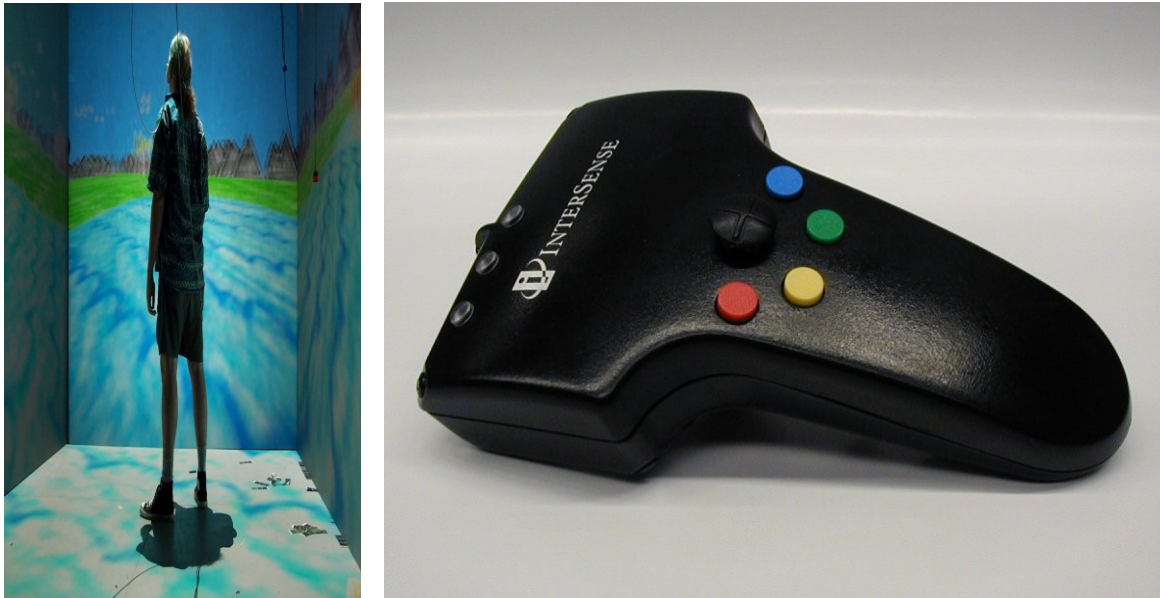
Figure 3 - left: a user interacting with CAVE; right: a wireless wand used as the input device for CAVE. Images from (left to right): https://www.lifehack.org , https://cosmosmagazine.com
