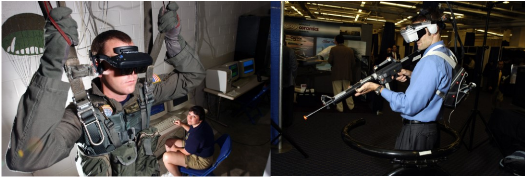
Figure 4 - left: a military parachuter in VR training environment, using parachute straps as the input device; right: a user in shooting training session with a model gun. Images from (left to right): http://www.vrs.org.uk , https://en.wikipedia.org
