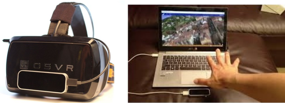
Figure 6 - the Leap Motion USB-like device. Left: mounted on a VR device; Right: used in a desktop environment. Images from (left to right): https://en.wikipedia.org , http://smartgimmick.com
