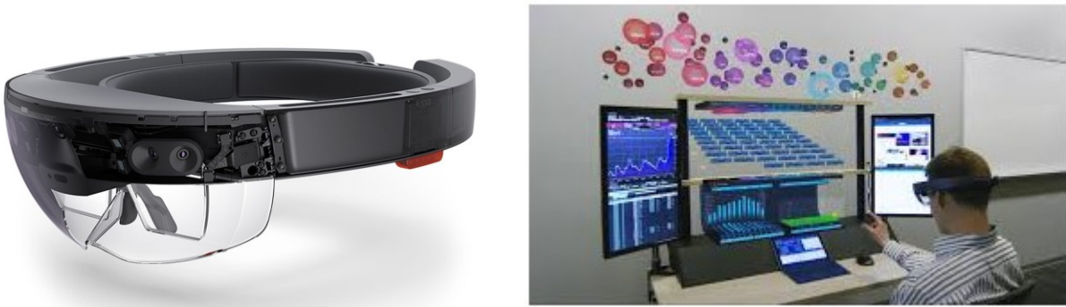
Figure 7 - Microsoft HoloLens, with voice and gesture recognition built in. Right: a HoloLens-wearing user issuing gesture commands in front of mid-air hologram charts. Images from (left to right): https://www.microsoft.com/en-ca/hololens , https://sg.news.yahoo.com/
