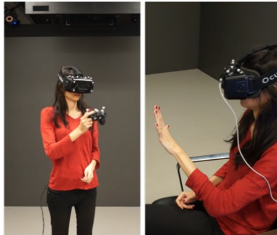
Figure 9 – Mota et al. 's study comparing gamepad and gesture inputs. On the left: user with a gamepad; On the right: user interacts with an Oculus Rift where a LeapMotion sensor was attached. Images from: [6]
