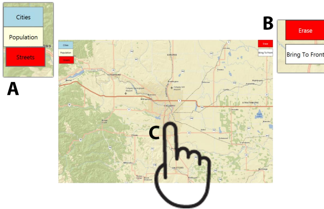
Figure 4.9 Users interact with lenses through (A) the lens selection menu, (B) the operations menu, and (C) touch gestures.
