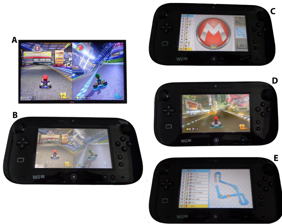
Figure 2.12 Wii U integrated with a TV. (A) TV displaying two players; (B) controller displaying the same information as TV; (C) menu to change the content displayed on controller; (D) controller showing only the player’s view; (E) controller displaying an overview and additional information of the race.
