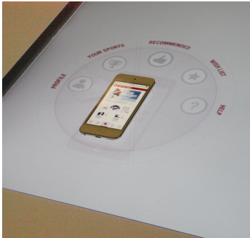
Figure 1. Personalized phone menu that appears when a smart phone device is placed on the tabletop.
