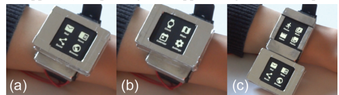
Figure 11. Launching apps: (a, b) frequent app icons in left and right groups; (c) viewing more app icons in group.
