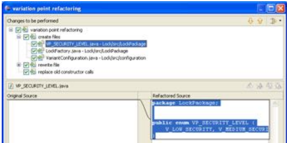
Figure 51 - The developer is made aware of the refactoring steps and the potential changes to the code
