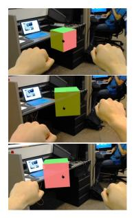
**Figure 2.** Real-time use of the Kinect in coordination with the HoloLens. Similar to Figure 1 except that the gesture is used to rotate the cube rather than enlarge it
