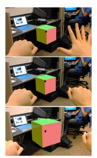
**Figure 1.** Real-time use of the Kinect in coordination with the HoloLens. In frame one, the user anchors the object by closing one hand. In frame two, the user positions his second hand in order to calculate relative distance between hands. In frame three, the user enlarges the object by widening his hand position.
